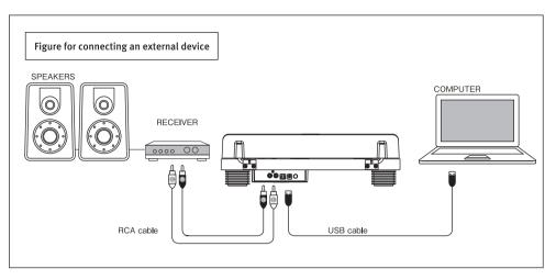
This product is equipped with a built-in speaker. Please refer to the above diagram if you connect your external speaker to the record player. Insert an RCA cable (not provided) to the RCA output jack, then connect to your external speaker.
